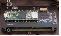
Use 4 of the included ABS spacers (black) to space TD1220RDR away from bezel as shown. You can use craft paste (or other light adhesive) to hold upper two spacers in place during assembly. The lower two spacers can be held in place with screws since TD1220RDR uses open slots for lower two mounting points.
